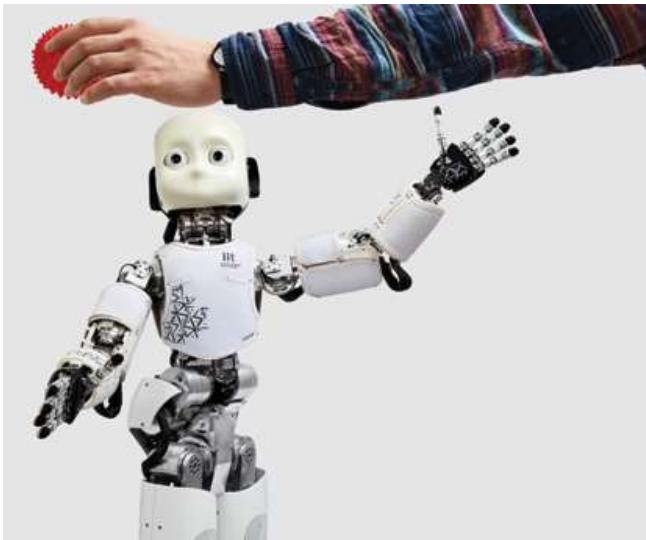
ICUB, an android being studied at the University of Plymouth in England, can learn new words, such as “ball,” more easily if the experimenter consistently places the object at the same location while naming it.
